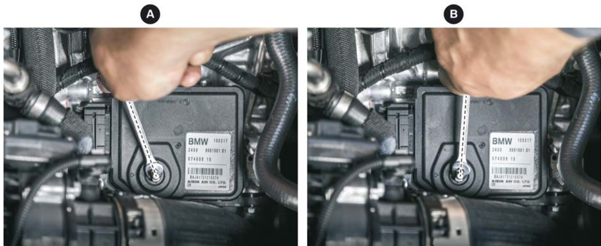
AISIN TU (8G45-460) Manual emergency release of parking lock
