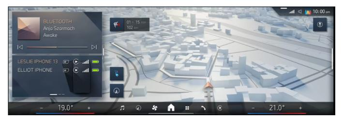
The Home Screen concept has been upgraded. All widgets have been relocated to the left side of the Home Screen Stage into the QuickSelect Menu. The widgets can be moved up or down in the QuickSelect Menu to access other widgets that are off-screen. This allows for quick access to all information without blocking the display on the Stage.
